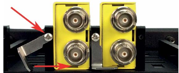
Modules are clamped securely into position
