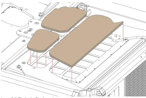
Image 2–3 Placing the filter foam pieces
