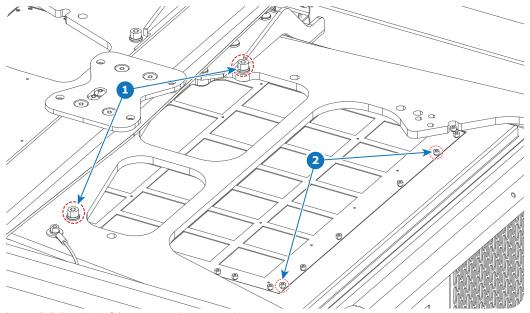
Image 2-2 Location of the screws to be removed
