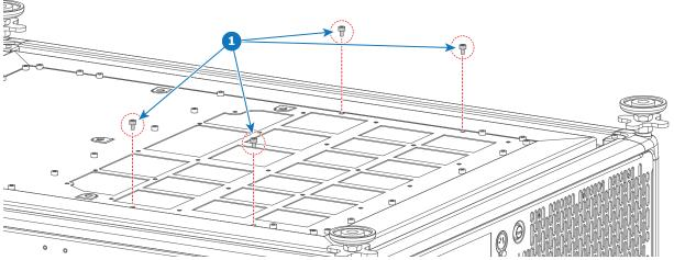
Image 2-5 Screws from the bottom plate to be removed
