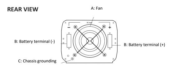
A: Fan: Do not obstruct, allow at least 12 inch for air flow.
