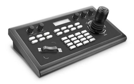
A network (IP Based) PTZ camera controller, is fully compatible with many PTZ camera coding protocols from the main manufacturers in the market, supporting ONVIF, VISCA, Serial port VISCA, PELCO-D/P protocols and etc. This compact camera controller features a high-quality joystick that allows variable speed control, as well as fast camera switching, quick-set camera parameters and so on. The industrial-grade blue screen LCD module has excellent display effect with fine and clear characters.
