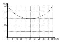
Figure 1 Relative Humidity Accuracy
