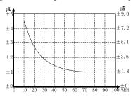
Figure 3 Dew Point Accuracy (at 25°C)
