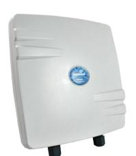
The NetWave® NW10[E] Industrial Grade high performance wireless radio is ideal for high capacity and scalable deployments where channel overlapping and interference typically cause our discounted competitors radios to become unstable. The wide range of channel spectrum widths available on the NW10[E] series of radios gives you the option of narrowing channel bandwidths as your network grows which will increase the number of non-overlapping channels and improve stability.
