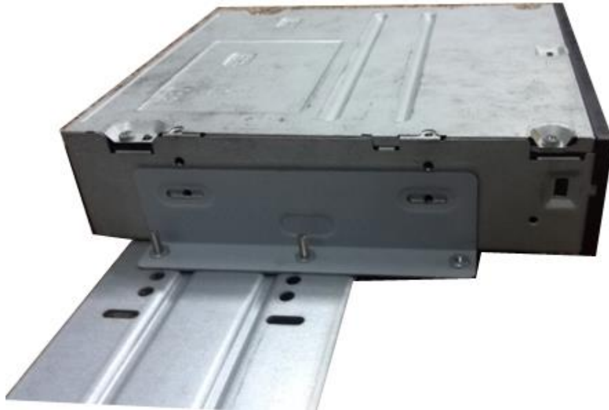
Figure 3-43 Install SATA burner
