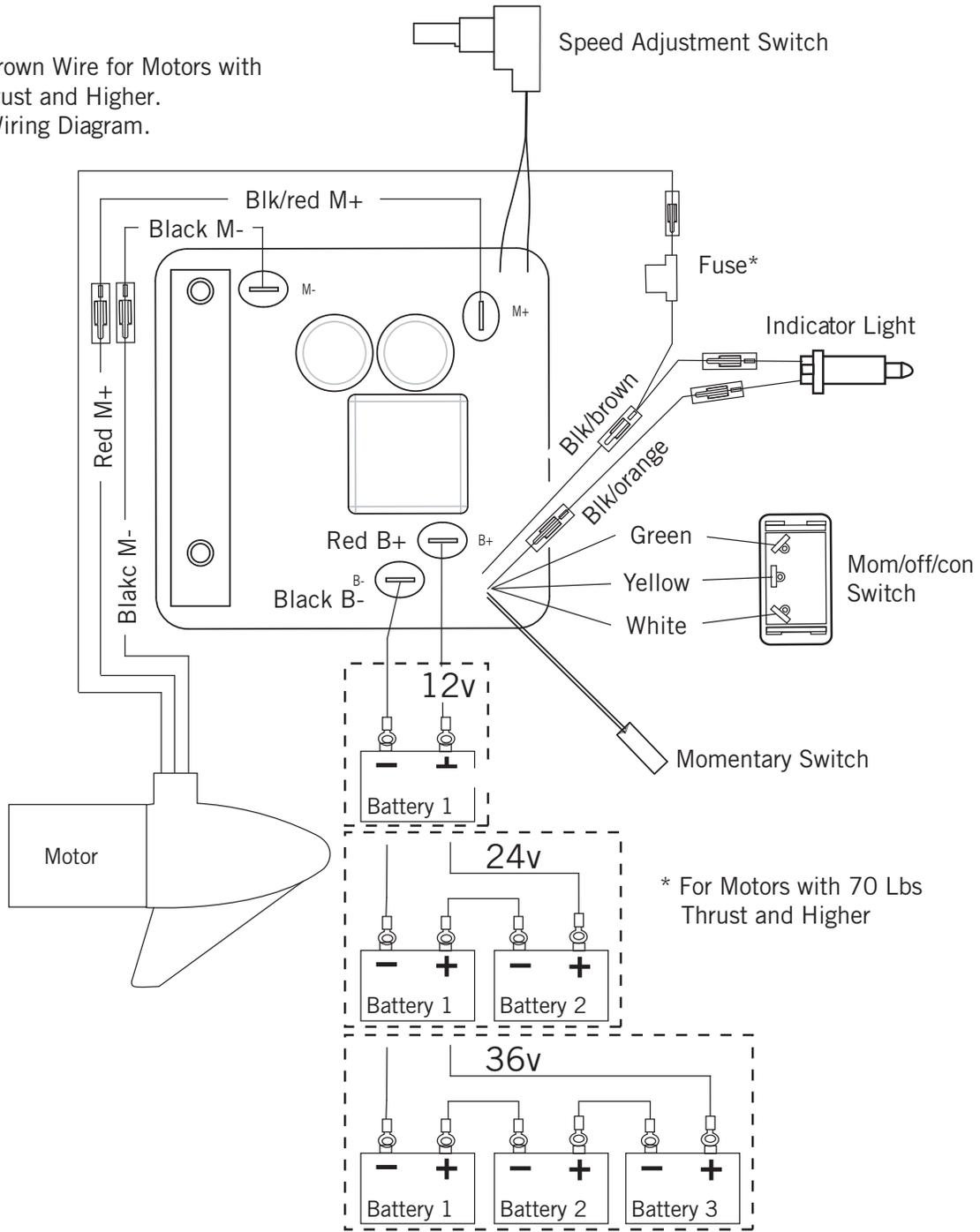
**NOTICE:** This is a multi-voltage diagram. Double-check your motor's voltage for proper connections. Over-Current Protection Devices are not shown in this illustration.
