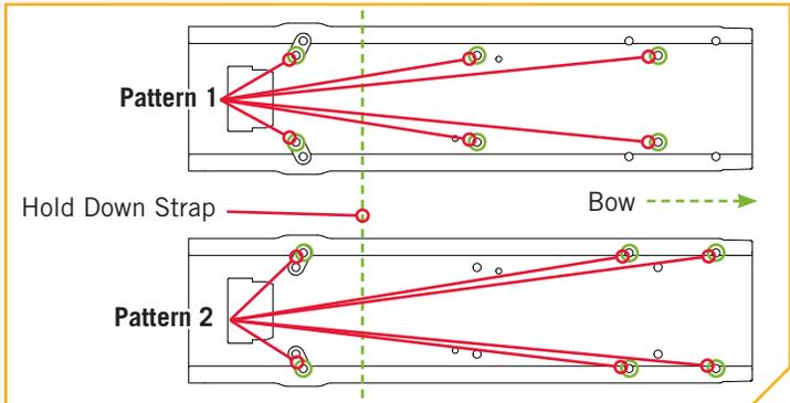
**NOTICE:** To prevent seizing of the stainless steel hardware, do not use high speed installation tools. Wetting the screws or applying an anti-seize may help prevent seizing.
