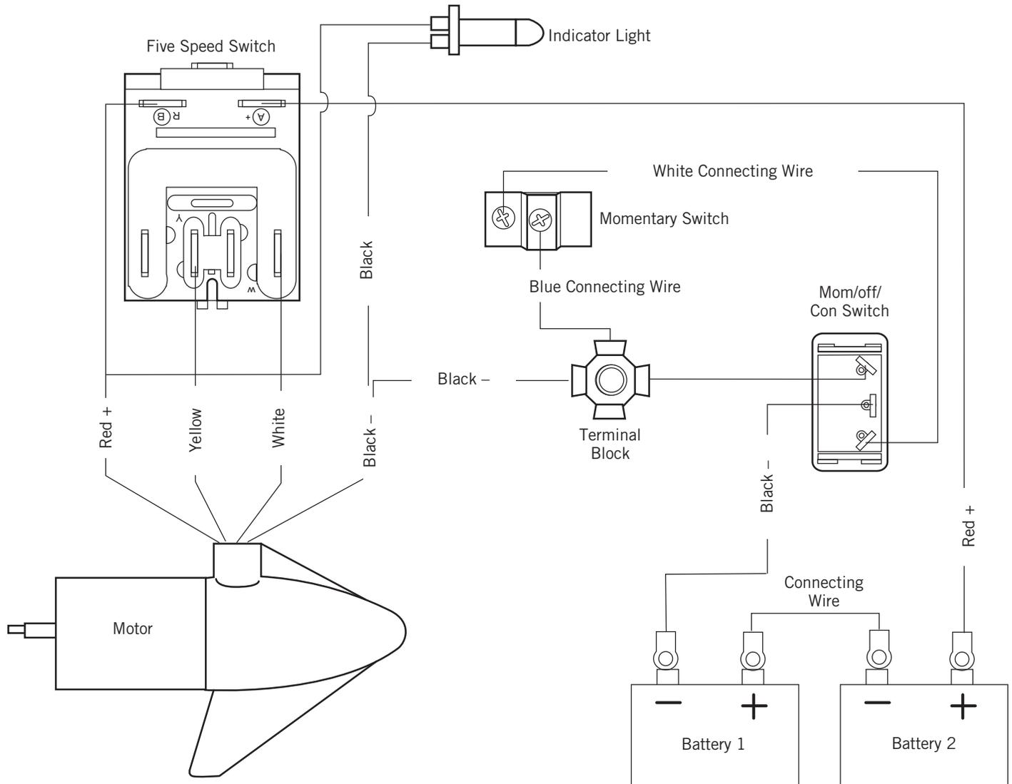
**NOTICE:** This is a multi-voltage diagram. Double-check your motor's voltage for proper connections. Over-Current Protection Devices are not shown in this illustration.
