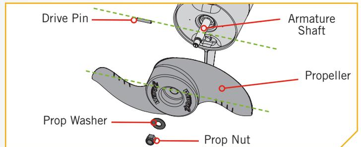
**NOTICE:** If the Drive Pin is sheared or broken, you will need to hold the shaft stationary with a flat blade screwdriver pressed into the slot on the end of the shaft while you loosen the Prop Nut.
