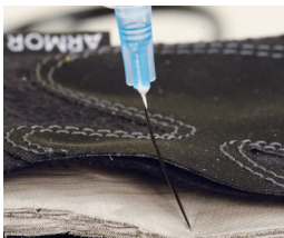
25 gauge needle buckling
