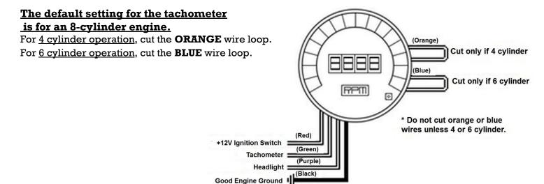
Ground - Black Connect directly to the engine block.
