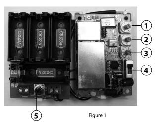
trol (Figure 1-5). This can be used to increase or decrease the sensitivity of the probe. In most locations the sensitivity should be set at the mid point (12 o'clock). Rotate the knob clockwise in one hour increments to increase the sensitivity. Note, do not operate with the sensitivity knob fully clockwise, as false signals may result. Move the knob slightly off the fully clockwise stop.
