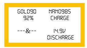
If the battery pack is deemed "Smart" (communicates with the charger based on various installed protocols), the top line will display battery name. If the pack is not communicating smart battery data, then the charger will display battery voltage. The lower line displays charging status.
