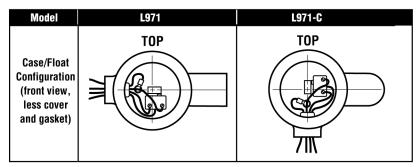
**NOTE:** Switches shown tripped on falling level.
