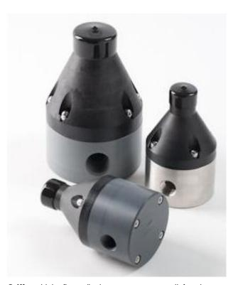
**Griffco** high flow diaphragm pressure relief valves are designed to protect chemical transfer systems from over pressure damage caused by defective equipment or a blockage in the chemical line. Large orifice sizes facilitate high flows and high viscosity. Wetted materials include **PVC**, **CPVC**, **PP**, **PVDF**, **PTFE**, **316SS**, **A20** and **Hast**. **C**. Available sizes: 1/2", 3/4, and 1".
