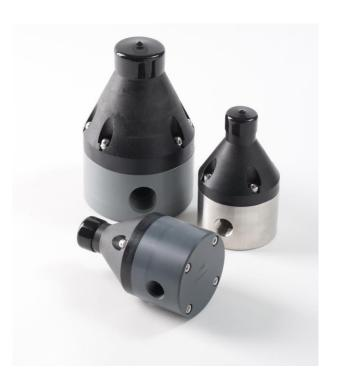
**Griffco** high flow diaphragm back pressure valves are designed to enhance the performance of higher flow, continuos feed pumps that require a constant head pressure, while also acting as an anti-syphon valve. Larger orifice sizes make the valve ideal for use with higher viscosity fluids. Wetted materials include: **PVC**, **CPVC**, **PP**, **PVDF**, **PTFE**, **316 SS**, **A 20 and Hast. C**. Available in 1/2" – 2" sizes.
