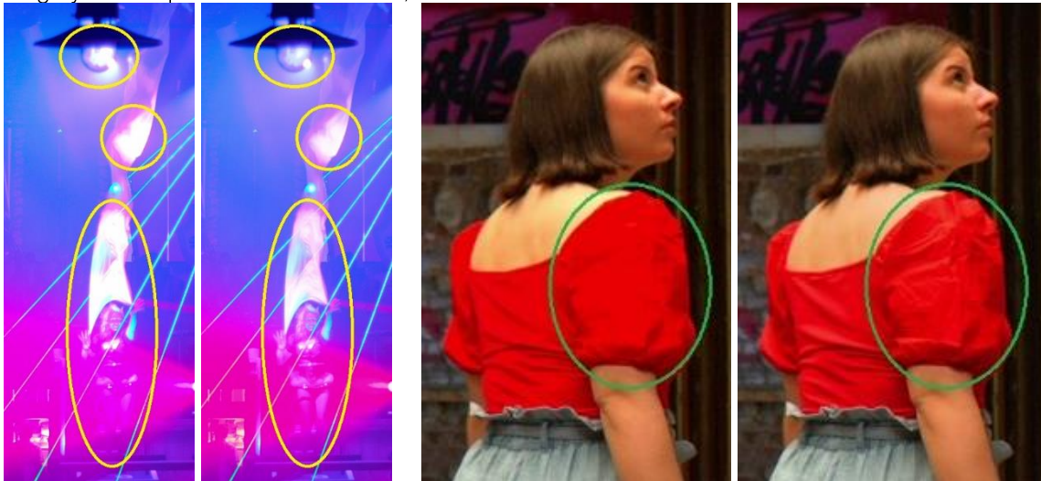
Clipping of the color values (left) vs. Mapping of the color values (right)
