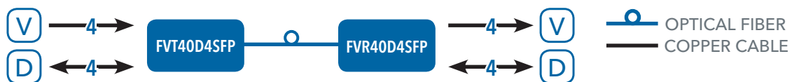
Optic Fiber Count and Type dependent on user selection of SFP modules.
