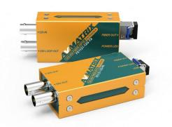
The FE1121-12G 4K 12G-SDI Fiber Optic Extender is a transmitter/receiver kit supporting single-mode LC simplex fiber extensions up to 10km. It is a miniature-style extension solution that supports all SDI formats resolution up to 4K with audio and metadata. It features a local SDI loop out and dual SDI outputs and supports 12G/6G/3G/HD/SD-SDI signals.
