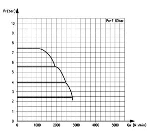
ER204-9xxx Flow characteristics Pr = output pressure (bar) Qn = flow (l/min) Pa = working pressure (bar)
