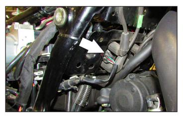
5 Plug the DRL-400 in-line of the stock wiring harness and ignition coil.
