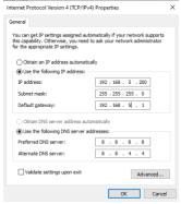
**NOTE:** When you are finished configuring the camera you will need to return to this screen and click the bubbles for "**Obtain an IP address automatically**" and "**Obtain DNS server automatically**" to restore internet connectivity to your computer. Also make sure to reconnect any ethernet cables you may have unplugged.
