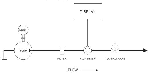
Install the meter upstream from control valves and fluid regulators if possible. Back pressure from control valving is beneficial for stable running.
