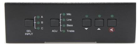
The SEL INPUT button and A/B/C LED indicators select which line input on the rear panel is mixed into the MIC INPUT, RCA, 3.5mm or SPDIF inputs respectively.
