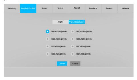
VGA output resolution can be selected as 1024x768@60Hz, 1280x720@50Hz, 1280x720@60Hz, 1360x768@60Hz, 1600x1200@60Hz, 1920x1080@50Hz, 1920x1080@60Hz (Default) or 1920x1200@60Hz.
