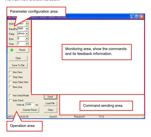
Please set the parameters of COM number, bound rate, data bit, stop bit and the parity bit correctly, and then the command is ready to be sent in command sending area.
