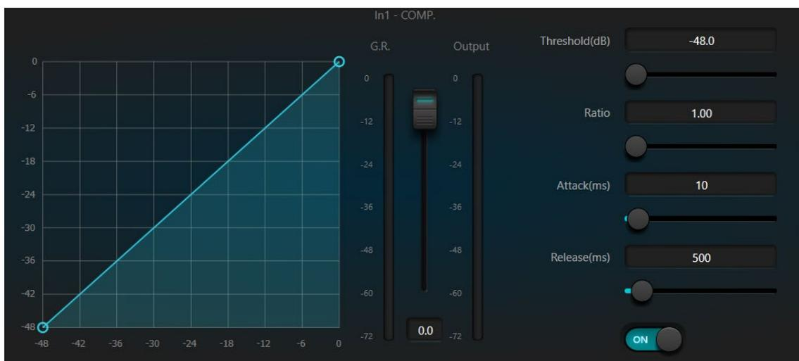
**Threshold:** When the signal level is higher than the threshold, the compressor / limiter begins to reduce the gain. Any signal that exceeds the threshold is regarded as overshoot signal, and its level will be reduced based on the ratio set. The more the signal level exceeds the threshold, the more level is attenuated.
