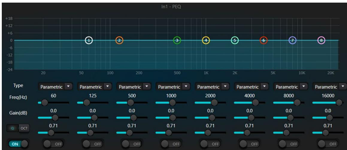
The equalizer has the following control parameters:
