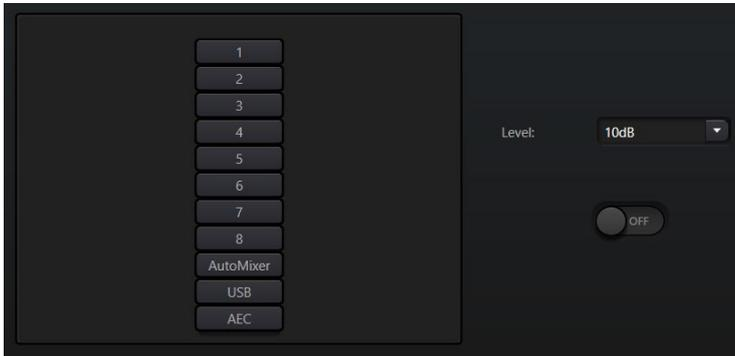
**Suppression level:** There are three levels of noise suppression including: Mild (-6dB), Medium (-10dB) and Aggressive (-15dB). dB here refers to the reduction in decibel level of the suppressed noise. The bigger the value, the more degradation of voice signal is caused, therefore use noise suppression very cautiously.
