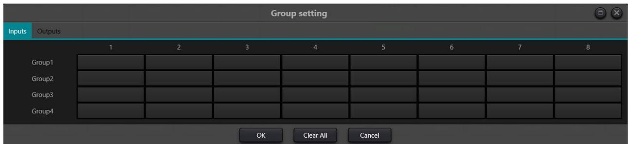
There are 4 groups in total. 1-device maximum number of channels can be selected for each group. The maximum number of channels is determined by the device type you purchased. Channels are set into one group which will be differentiated by a color difference of the volume slider in the main interface.
