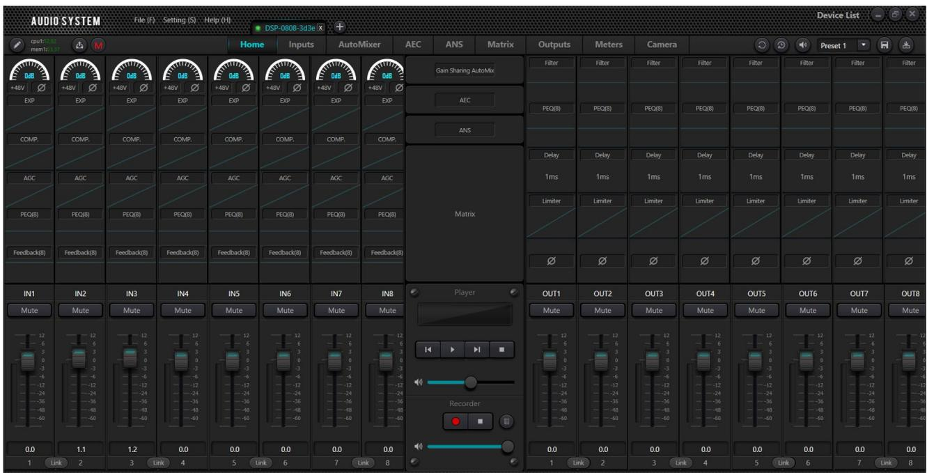
Click the button
