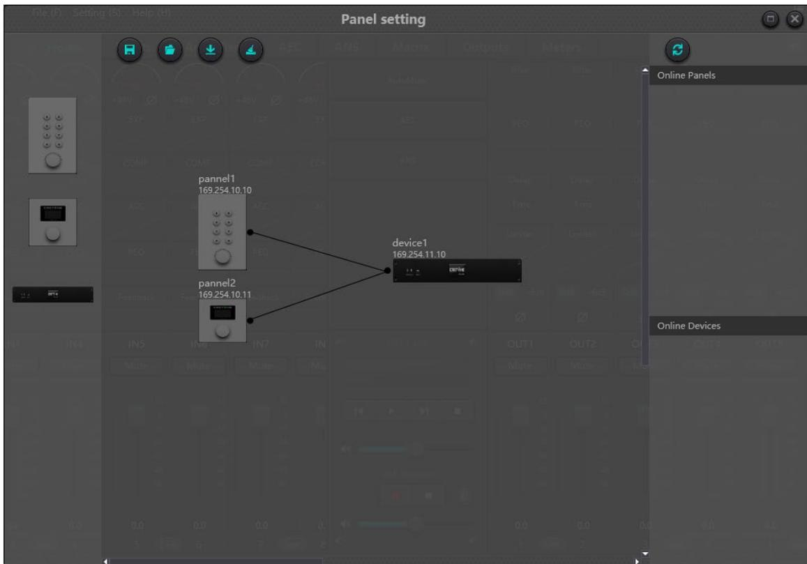
**Offline device:** In offline edit status, the commissioning engineer configures the panel parameters locally, and then downloads it to the online panel. The panel can then be edited directly online. Drag an offline device from the column of online panels to the panel design area and then double click to edit it.
