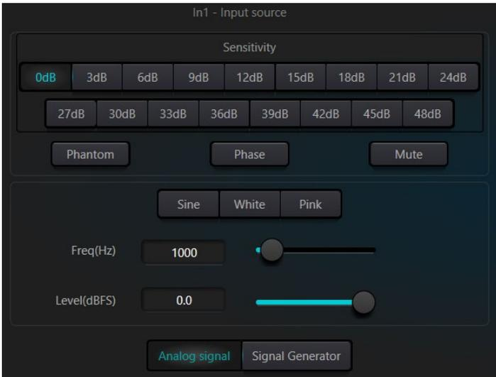
**Sensitivity:** Microphone gain, 0dB - 48dB in 3dB Steps.
