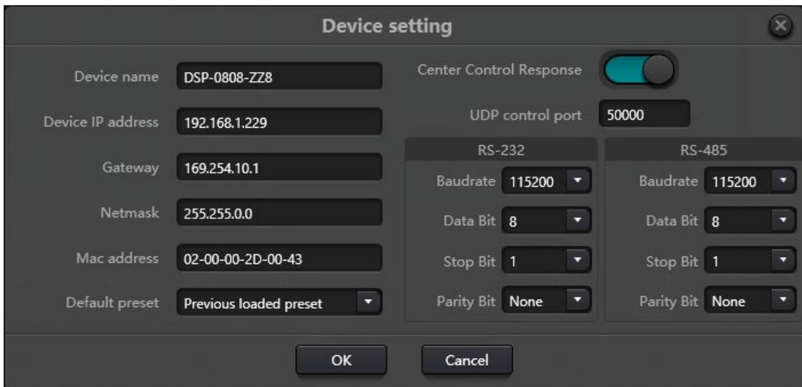
Information like device name, network address and serial baud rate can be set under device setting. The maximum length of the device name is 16 characters.
