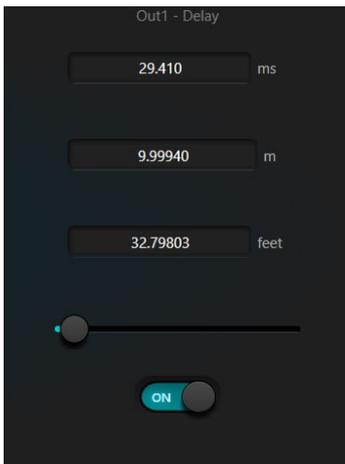
**Activate button:** Turns On / Off the delay module and inserts it into audio signal path to increase fixed delay time for signals.
