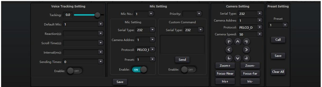
**Voice tracking threshold:** Detects a microphone input signal greater than or equal to the tracking threshold, the system will automatically enable tracking parameters when threshold is exceeded.
