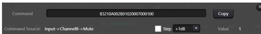
Open the central control command window and select the parameter to be controlled on the DSP GUI interface. The window will display the current command immediately. Copy the command and then use UDP or RS232 to send the command to the device form external control interface.
