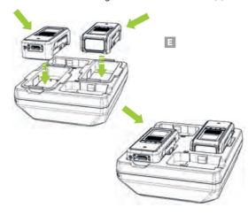
3. KDC185 Ring Trigger can now be charged while wearing a protective boot. Charge the device by placing the device on the cradle with the scan engine facing upward. (H)
