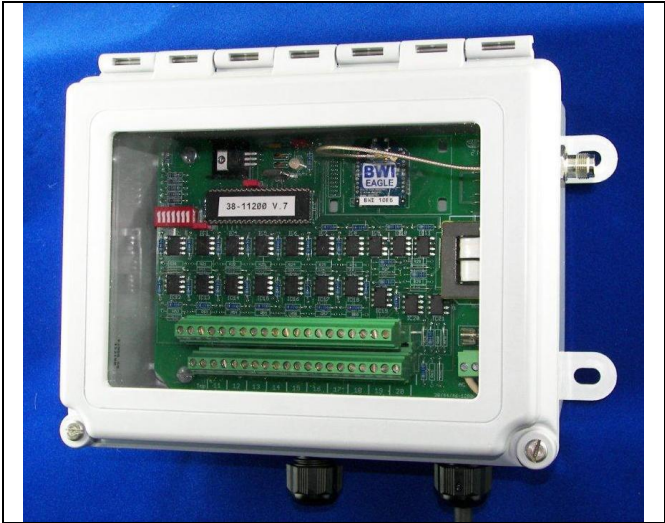
Note – AC powered model pictured Dimensions 8" L x 6" W x 4" H
