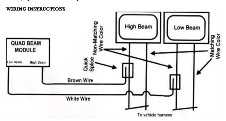
Note: Automotive circuit connectors are the preferred method of connecting wires, although you may solder if you prefer.
