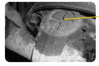
Fits in most Mack truck king pin caps to remove king pin. Designed to fit in the "+" design with precision
