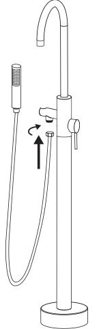
6. Install the hose to the handshower and the tub filler. Please check the tub filler spout and handshower water flow and its function.
