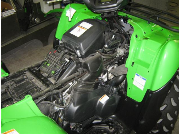
Picture 1: Remove the engine covers Exposing the frame, coils and wiring.
