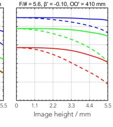
– 20 LP/mm, radial 40 LP/mm, radial 80 LP/mm, radial --- 20 LP/mm, tangential --- 40 LP/mm, tangential --- 80 LP/mm, tangential
