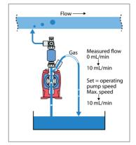
After the gas has been purged, the EFS sensor will begin to measure flow. Feedback from the sensor controls the pump, slowing it back down so the flow rate meets the set
