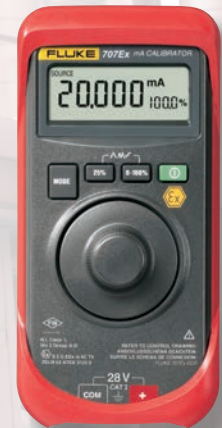
Fluke 707Ex Loop Calibrator
