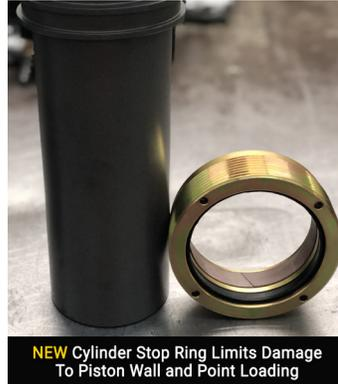
The first-generation cylinder stop ring had a single groove machined for the piston rod wiper. The wiper kept internal contamination to a minimum, as was designed, it also created a slight side to side movement. This movement increased point load situations which, in turn, caused severe scarring on the outside walls of the piston rod as well as the internal walls of the cylinder.
