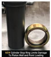
The first-generation cylinder stop ring had a single groove machined for the piston rod wiper. The wiper kept internal contamination to a minimum, as was designed, it also created a slight side to side movement. This movement increased point load situations which, in turn, caused severe scarring on the outside walls of the piston rod as well as the internal walls of the cylinder.
